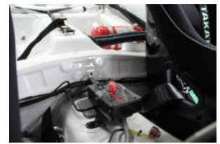
Automatic fire extinguisher
