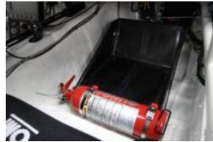
Co-Driver footrest & handheld Fire Extinguisher
